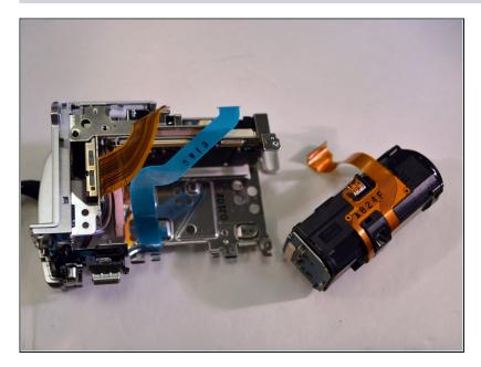
• With the old lens module removed, the new one can be installed.
