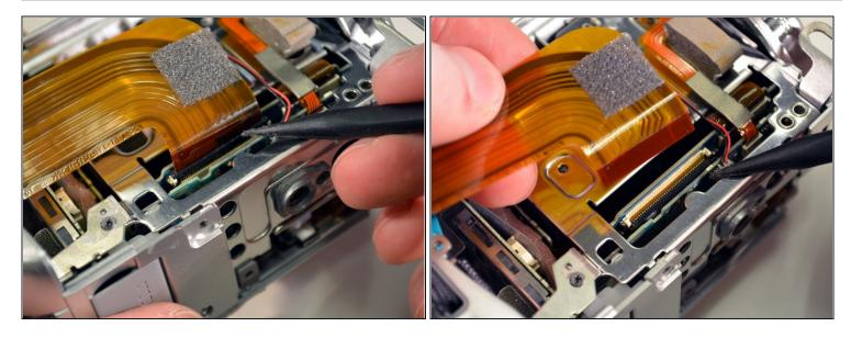
• Using the pointed black spudger, carefully open the little black clasp on the large ribbon wire port.
