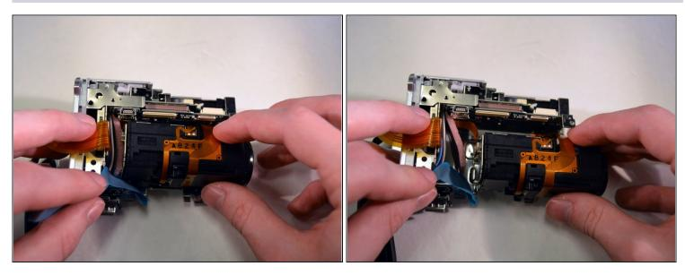
i The lens module is connected to the device by an adhesive foam backing.
