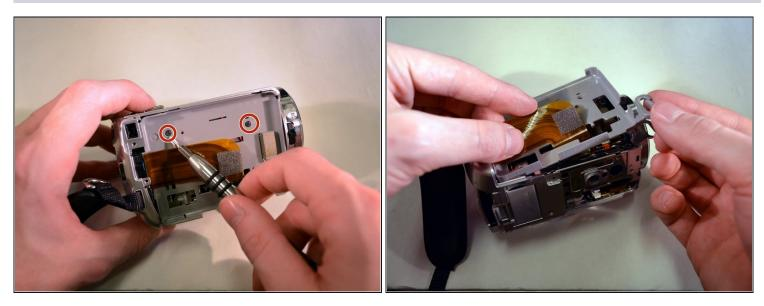
• On the right side of the device, remove the two black 3mm Philips screws.
