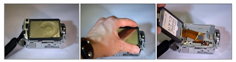
• Using your fingers, lift the HDD from its right end, pivoting on its left end.
