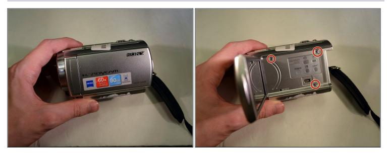
• On the left side of the device, remove all visible 3mm Philips screws.
