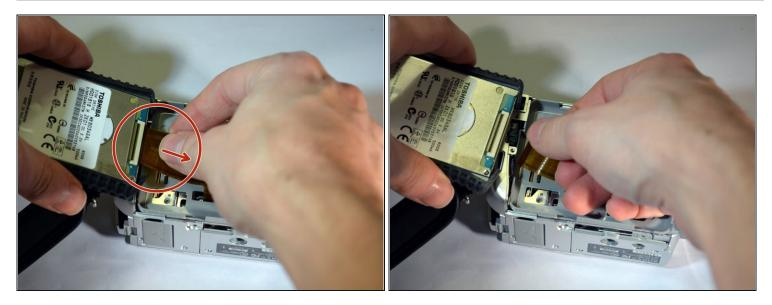
• While securely holding the HDD in your left hand, use the soft pad of your right hand fingers to gently pull the ribbon wire out of its socket, toward your right.
