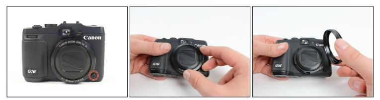
• Remove the ring around the lens by simultaneously pressing the black button located at the bottom right of the ring and rotating the ring counterclockwise.
