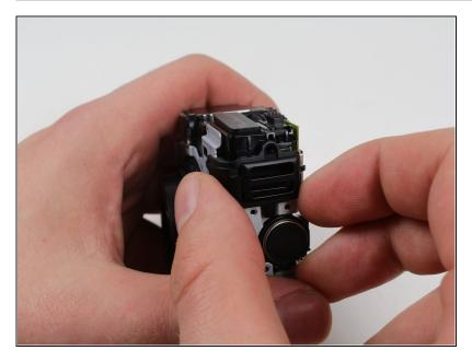
• Remove the cable strap bracket by lifting it away.
