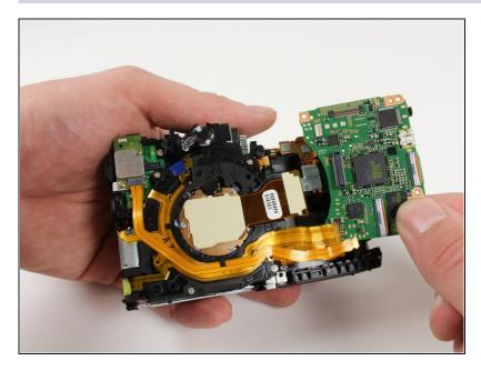
• Lift the motherboard out of the camera.
