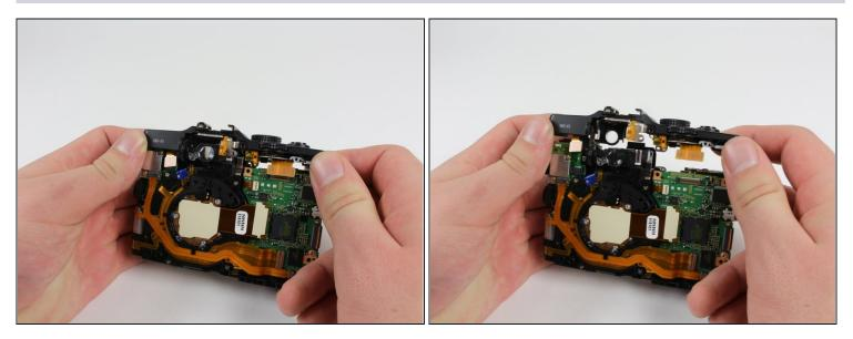
• Remove the top portion of the casing by firmly grasping it and pulling it upward to lift it off.
