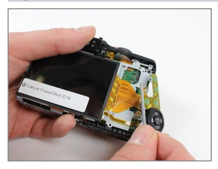
• Lift the button circuit board away from the camera.
