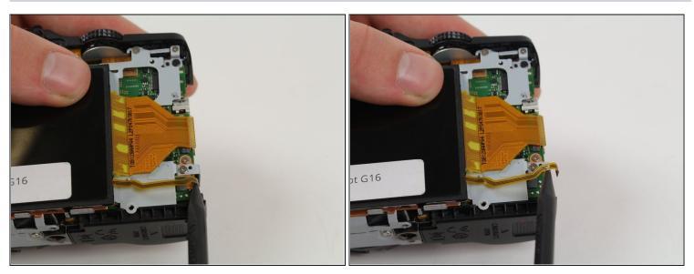
• Unplug the small connector ribbon by pulling the cable outwards from the camera using a spudger or your fingers.
