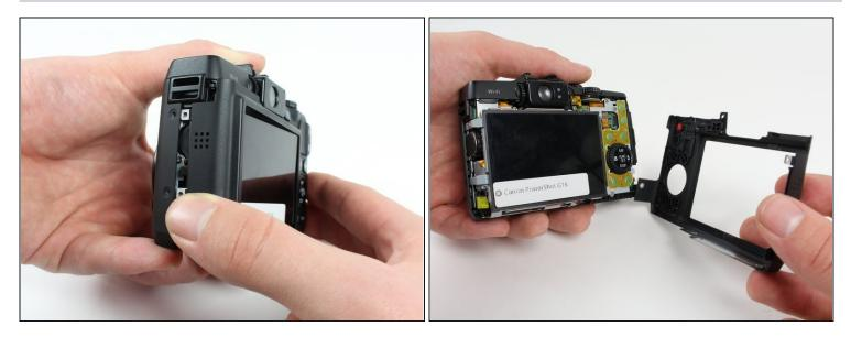
• Using your fingers, carefully pull the the back cover off by grabbing the bottom left of the back cover and pulling outwards.
