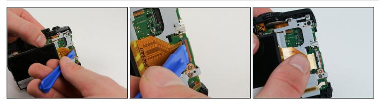
⚠ Do not pull the connector upwards as doing so may harm the connector housing.
