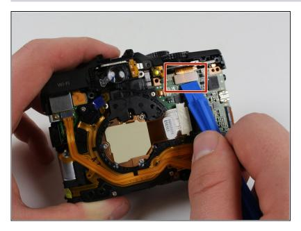
• Disconnect the cable on the top of the motherboard by lifting it up vertically using a plastic opening tool.
