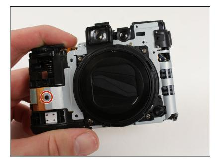
Remove the black 3.8 mm screw on the far left side using a Phillips #000 screwdriver.
