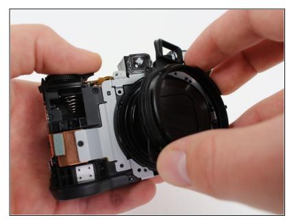
• Remove the black plastic cover surrounding the lens by gripping and lifting upwards.
