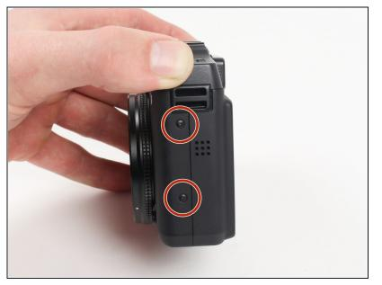
Remove the two 3.3 mm screws near the speaker using a Phillips #00 screwdriver.
