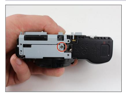
Remove the 2.7 mm screw from the bottom of the camera using a Phillips #00 screwdriver.
