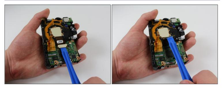
• Disconnect the lens cable from the motherboard by lifting it up vertically from the motherboard using a plastic opening tool.
