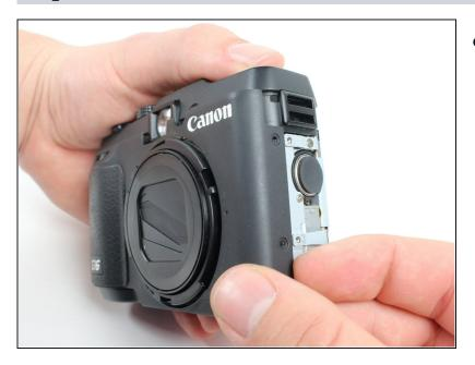
• Using your fingers, carefully pry the front cover off starting at the bottom right.
