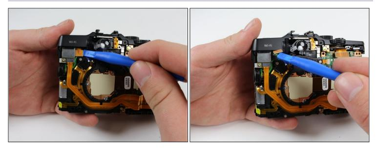
• Disconnect the cable on the back of the camera to the left of the viewfinder by lifting it up vertically using a plastic opening tool.
