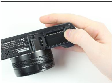
Flip the inside switch up to release the battery.
