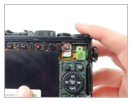
Use a Phillips #000 screwdriver to remove the 7.5mm screw on the top right of the back of the camera that holds the metal backing in place.
