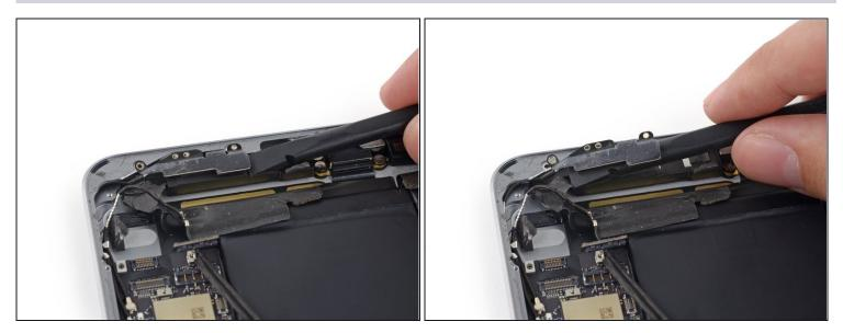
• Use the flat end of a spudger to cut the foam adhesive securing the antenna to the right speaker.
