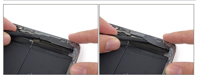
• Use the flat end of a spudger to loosen the foam adhesive securing the Wi-Fi antenna to the left speaker.
