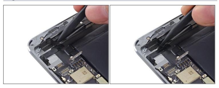
• Use the point of a spudger to separate the adhesive holding the antennas to the right speaker.
