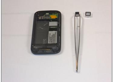
• Use the tweezers to pull the camera cover up and away from the phone. Repeat for the camera underneath.
