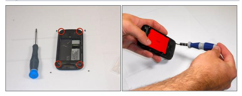
• Remove the four screws from the corners of the phone using a T5 Torx screwdriver.
