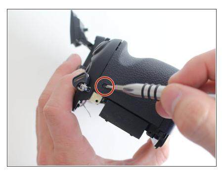
Remove the 5.0 mm Phillips #00 screw from the remaining leather material on the camera's side.
