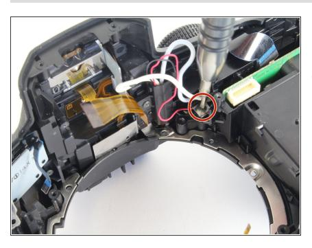
Remove the 5.0 mm Phillips screw from under the aperture mode selector.
