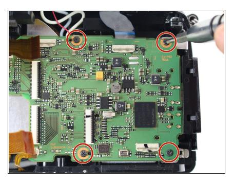
Remove the four 5.2 mm Phillips #00 screws at the corners of the motherboard.
