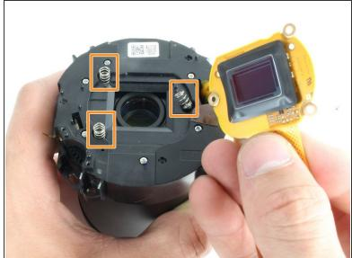
★ Keep the front of the lens face down. There are springs between the sensor and the lens which may fall out.
