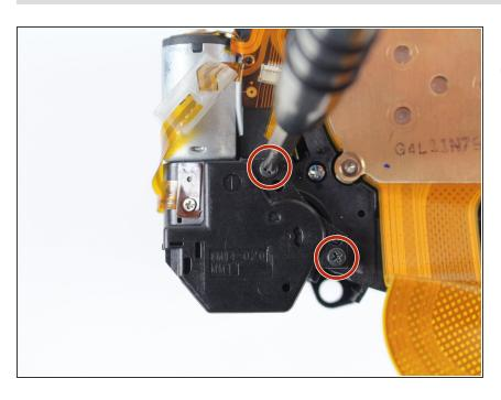
Remove the two 5.0 mm Phillips #00 screws near the lens on top of the aperture motor.
