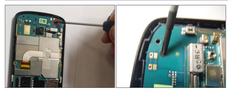
• Remove the single Phillips #0 screw that is securing the motherboard to the front case of the phone.
