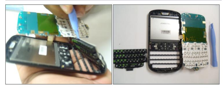
• Lift off main keyboard from front plastic case using plastic opening tool.
