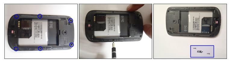
• Remove the six Torx #5 screws that are securing the rear frame.
