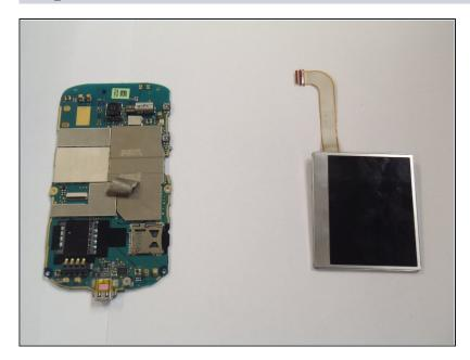
• Lift the Motherboard away from the LCD display.
