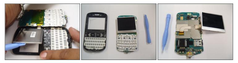
Remove the plastic cover from the LCD display and the motherboard.
