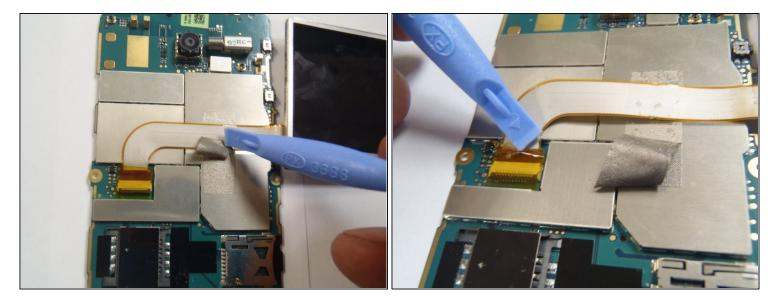
• Remove the gray tape securing the ribbon cable.
