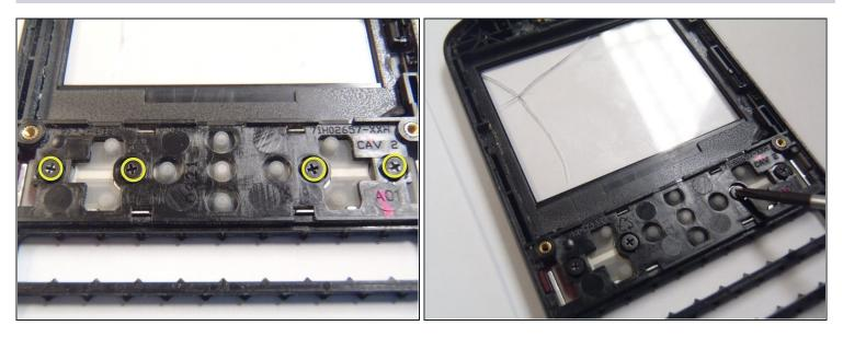
• Remove four Phillips #00 screws securing function keys.
