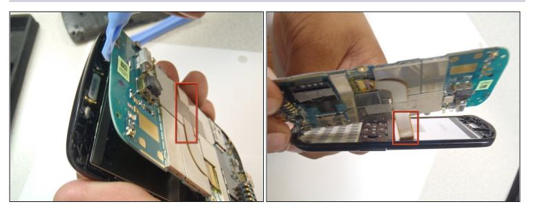
• Pry the motherboard away from the front of the plastic case using a plastic opening tool.
