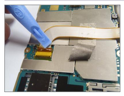
• Remove the yellow tape securing the connector lock.
