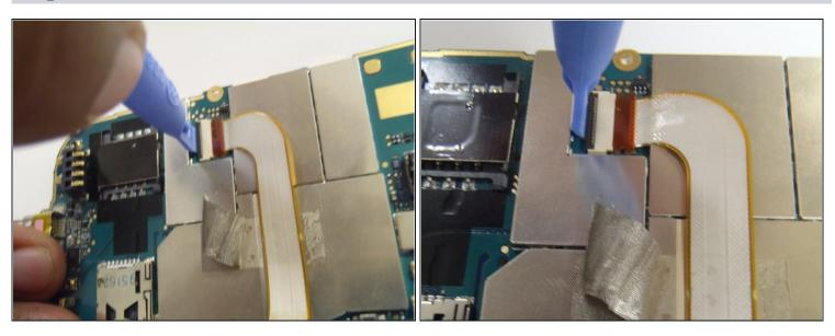
• Carefully lift the black lock to release the ribbon cable, using the plastic opening tool.
