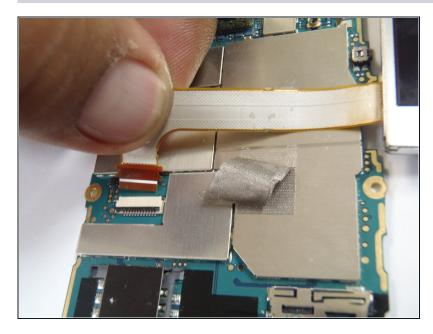
• Pull the ribbon cable upwards, disconnecting it from the Motherboard.
