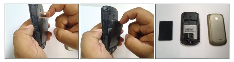
• Use your finger to push the top of the battery downwards and lift the battery out of the phone.
