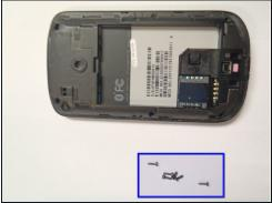
• Remove the six Torx #5 screws that are securing the rear frame.
