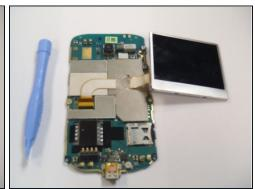
• Remove the plastic cover from the LCD display and the motherboard.
