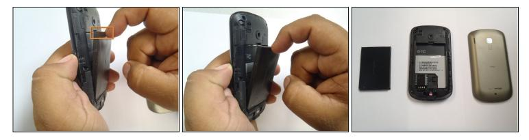
• Use your finger to push the top of the battery downwards and lift the battery out of the phone.
