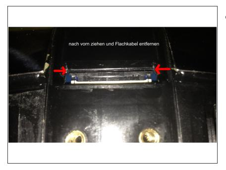
Carefully remove the ribbon (press the clamp still in front) and lay the docking arm to one side.
