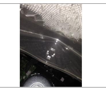
Use a flat plastic tool or a blunt knife in the slot between the chrome bar and speaker cover to push
