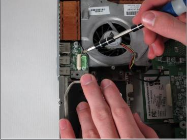
Unscrew the 6mm Philips screw connecting the USB module to the fan.
