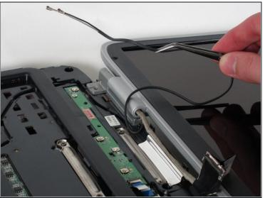
Using tweezers, pull the black cable towards the display and through the hole in the casing.
