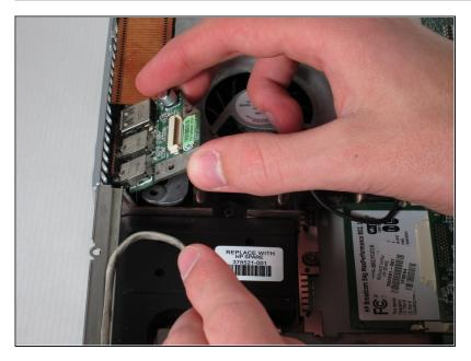
• Pull the module to the right and lift it out to release it.
