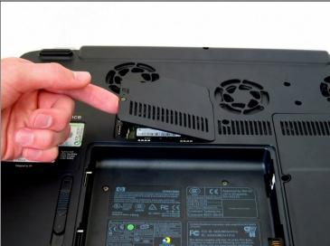
• Loosen the Phillips screw labeled 'ram' and lift the cover.
