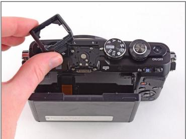
• Remove the external flash port casing to expose five more screws.
