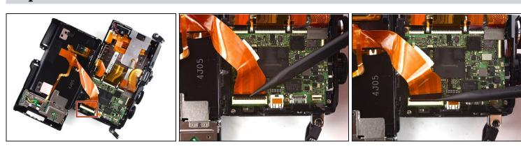
• To remove the ribbon holding the back case to the camera, use the pointed end of a spudger to flip back the top bar on top of the ZIF connector.
