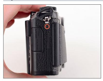
Use a Phillips #00 screwdriver to remove the 5 mm screw near the right hand grip.
