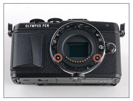
• Remove the two 4 mm Phillips screws.
