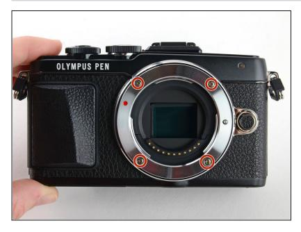
Use a Phillips #00 screwdriver to remove the four 6.3 mm screws from the lens mount.
