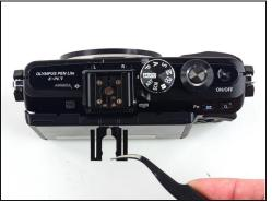
• Use tweezers to remove the metal clip from the external flash mount.
