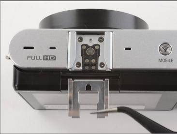
• Use <u>tweezers</u> to remove the metal shield from the external flash mount.
