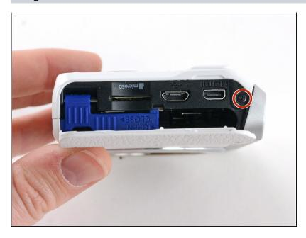
Use a Phillips #00 screwdriver to remove the 4 mm screw inside the battery compartment.
