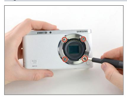
Remove the four 5 mm Phillips #00 screws from the lens assembly.
