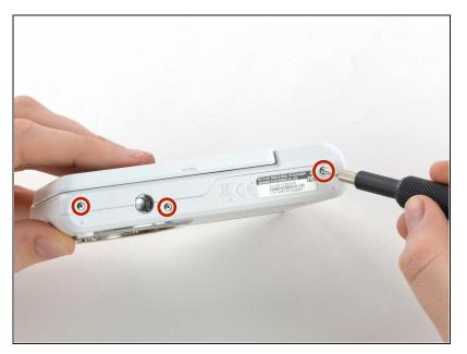
Use a Phillips #00 screwdriver to remove the three 4 mm screws from the bottom of the case.
