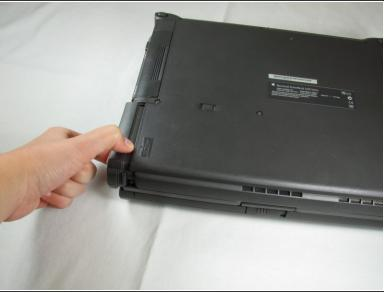
Hold the button on the front left side and slide the battery out.
