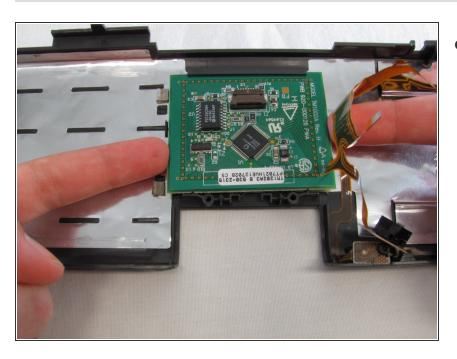
Remove the track pad by gently lifting up.
