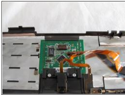
Push the buttons on the side of the ribbon cable port on the track pad to release the ribbon cable.
