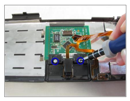
Remove two T8 7mm long torx screws from the bottom of the track pad panel.
