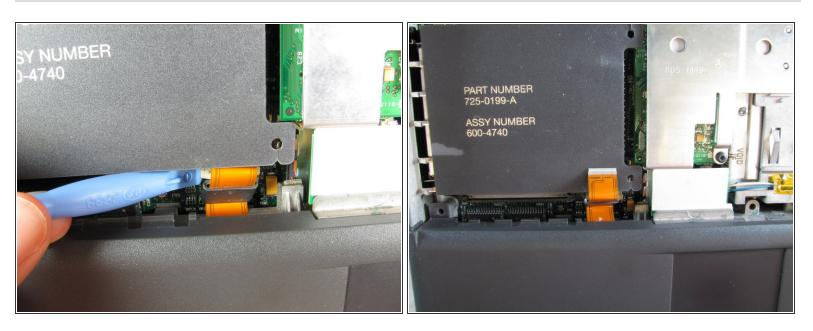
Use the plastic opening tool to lift up the tabs on either side of the ribbon cable port and then gently pull the ribbon cable free.
