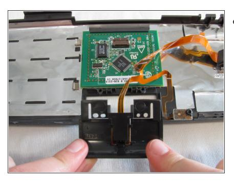
Slide the track pad button off of the track pad panel.
