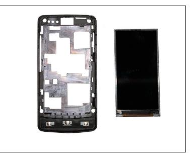
Simply lift the LCD screen from the logic board housing to remove the LCD screen.
