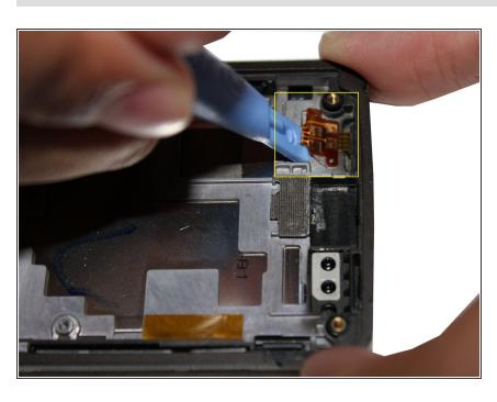
In the top right corner of the housing use a pry tool to disconnect the touch screen digitizer connector from the housing.
