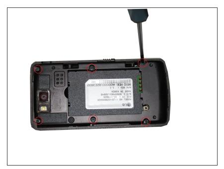
Six Phillips screws holding down the battery housing (Circled in the picture). Unscrew the six screws and put them aside.
