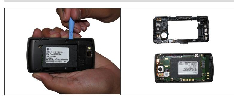
Insert a safe prying tool between the slot between the front screen housing and the battery housing to remove the battery housing.
