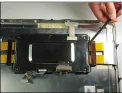
• Carefully remove the two tape plugs on either side of the control board using a spudger.
