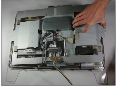
• Gently lift the large metal cover which spans across the back of the whole display.
