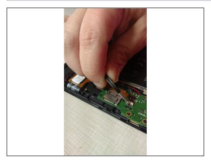
Using your fingernail or tweezers lift the holding flap and disconnect the digitizer cable for the old screen
