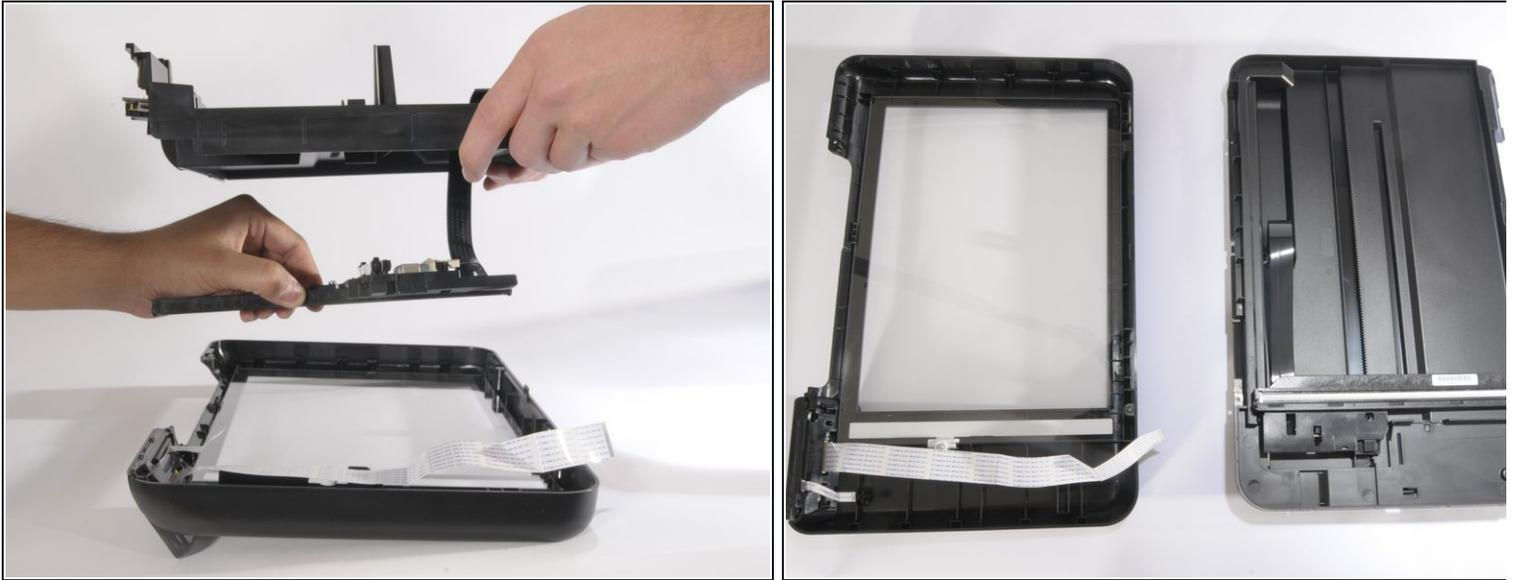
**⚠** Carefully separate the two hood pieces connected by the black ribbon.
