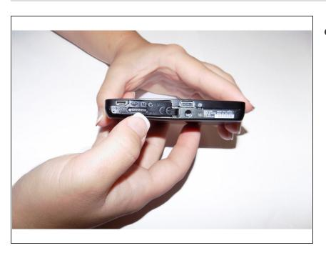
Slide the battery door in the direction that the arrows are pointing. The door will open outwards.
