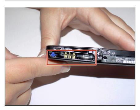
Slide the blue locking tab to release the battery. Slide the battery out of the camera.
