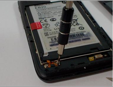
• Use the T-5 Torx bit to remove the two silver 3.3 mm screws with integrated washers.
