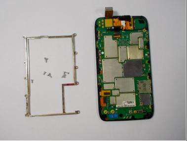
Remove the 10 Torx T5 screws, that hold the metal frame to the motherboard.
