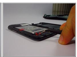
Remove the red rubber screw cover with a pair of tweezers
