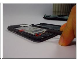
Remove the red rubber screw cover with a pair of tweezers
