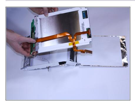
Remove the entire display EMI insulator from the casing.
