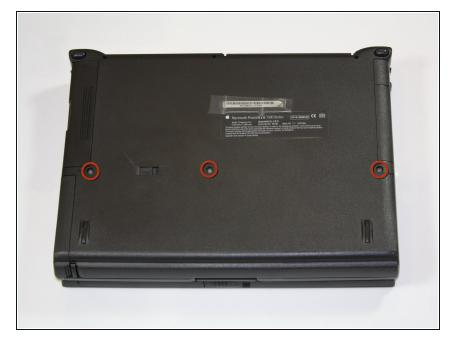
Turn the laptop over and remove the three T8 torx screws from the bottom panel.
