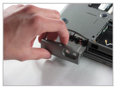
• Pull the hard drive tray directly away from the computer. The tray should slide out easily.
