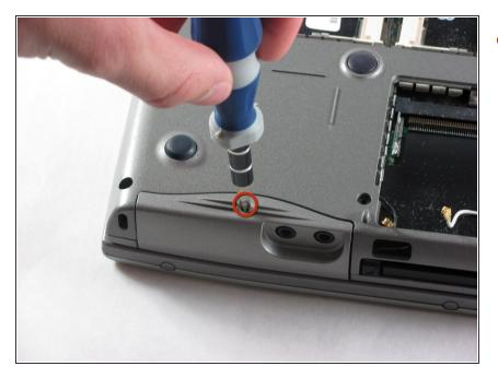
Use a #00 screwdriver to remove the single screw located in the center of the hard drive cover.
