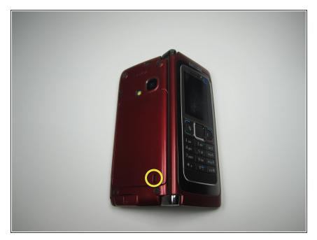
In order to remove the back cover, you must press the indicated button.
