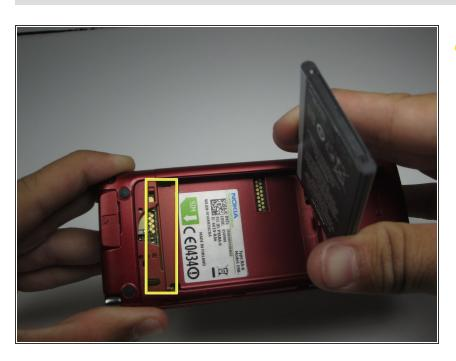
In order to remove the battery, pull it out from the same side that the rubber button is on.
