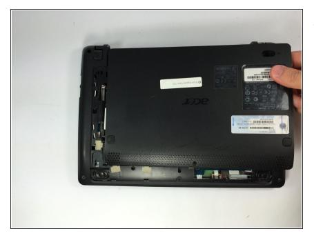
Gently lift up and pull away the backplate from the chassis to remove.
