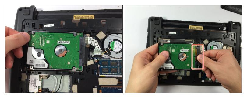
Gently lift and secure the HDD with one hand and carefully remove the SATA and power connections with your other hand.
