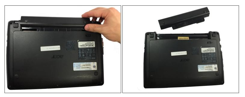
• If necessary, remove the old battery and replace it with a new one.
