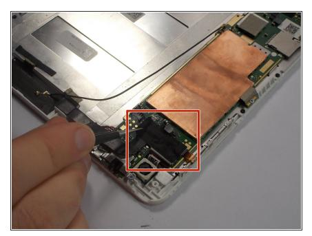
Remove the piece of black tape covering the rear facing camera ribbon cable connector.
