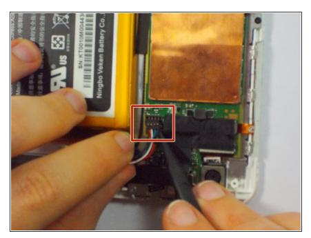
Remove the battery cable by lifting it up with the pointy end of the black nylon spudger.
