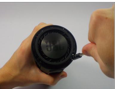
Remove the four screws that hold the passive radiator in place
