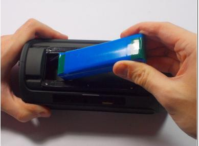
Use the plastic opening tool to remove the battery.
