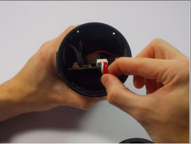
Remove the battery wire from the circuit board by pulling it out gently on the side closest to the LCD light.
