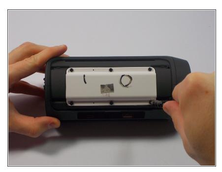
Remove the 6 screws that hold the white cover in place.
