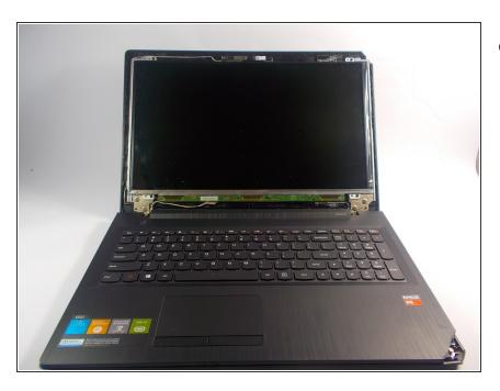
Test the new screen by turning it on before putting the bezel back on.
