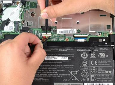
Press down on the white clip and softly pull the wires out of the port to disconnect battery from the motherboard.
