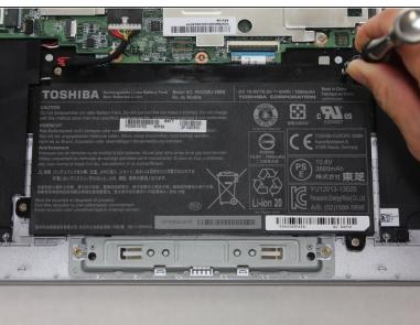
Remove the 4 Phillips 2 mm screws holding the battery in place with the Phillips #0 screwdriver.
