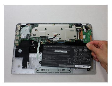
Remove the battery by gently pulling up on the bottom corners.
