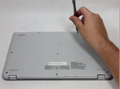
Remove the 8 visible Phillips 8.25 mm screws using the Phillips #0 screwdriver.
