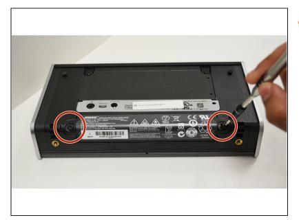
Using the screwdriver with the T-10 star tip, remove the 6.75 mm. screws marked in red.
