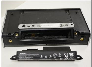
• Carefully remove the battery by pulling it out of the speaker.
