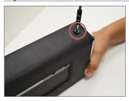
Using a 2.5 mm hex wrench, remove the two 13 mm screws from the bottom of the speaker.
