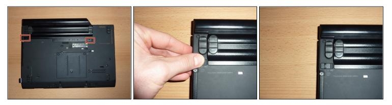
• Locate the two switches that lock the battery. Push the left-hand switch outward into the "unlocked" position.
