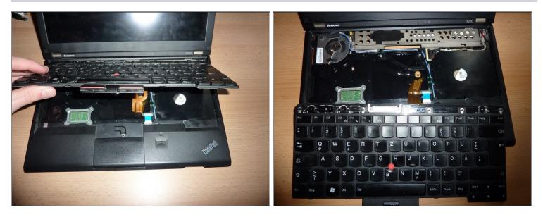
• Carefully lift the keyboard so that you can access its connector.
