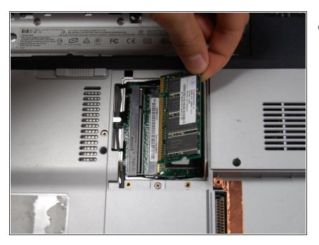
Gently lift the the RAM up and out of its seat.
