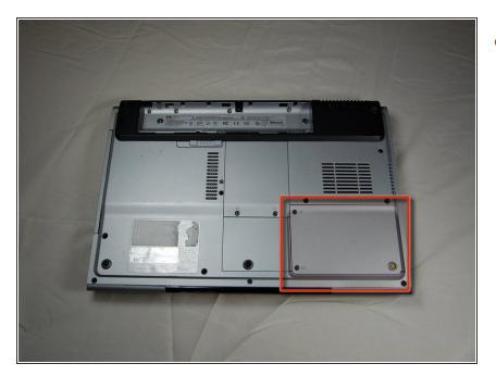
• With the battery removed, locate the hard drive access panel.
