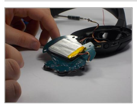
Gently removed and flip over circuit board to reveal battery pack attached to the underside. Careful not to pull out wires running through headband.
