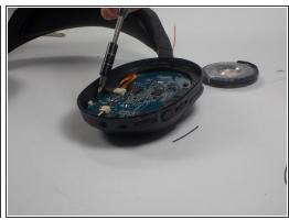
Use screwdriver tip J00 to remove three screws fastening circuit board to casing.
