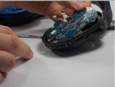
Circuit board will be free to be removed by hand. Use plastic pry tool to slide between casing and circuit board if needed.
