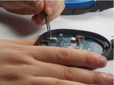
Use bent tweezers to remove two wire connector plugs from circuit board.
