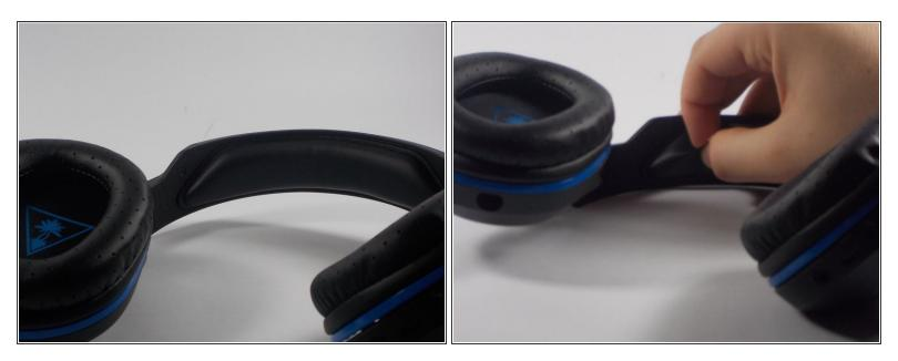
• Grab one end of the headband pad and pull up slightly, exposing where it is glued to to the backing.
