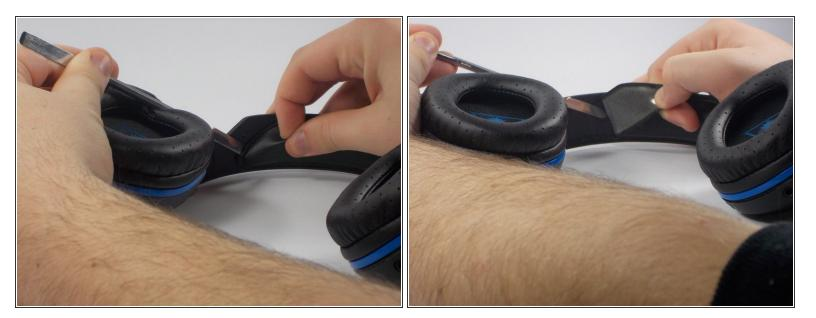
Using a thin tool carefully scrape away the glue underneath the band while pulling the pad up, careful not to rip it.
