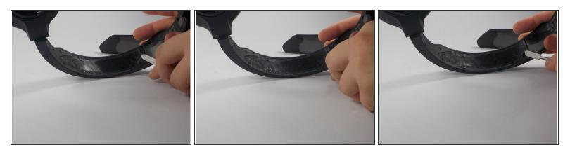
• Once the pad has been completely removed, scrape off any remaining residue.
