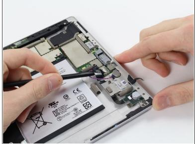
• Remove the silver bracket using the black pick in order to properly remove the entire audio jack.
