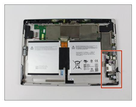
You will be working in this area of the Surface 3 when replacing the audio jack and Micro SD port
