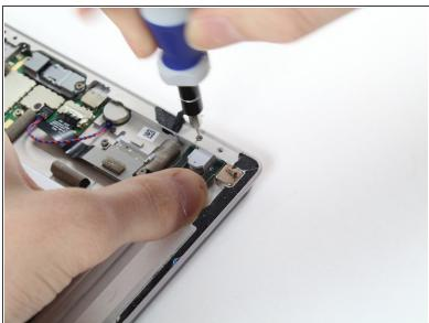
Remove the two 3/16" Torx #2 screws directly beside the audio jack.
