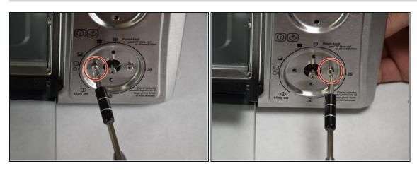
• Remove the two #2 Phillips Head x 5.5mm screws holding the timer controls to the face.
