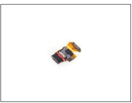
Push the charging port flex out of the slot and remove it.
