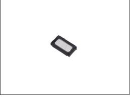
• Cut the adhesive underneath the earpiece and remove the earpiece.
