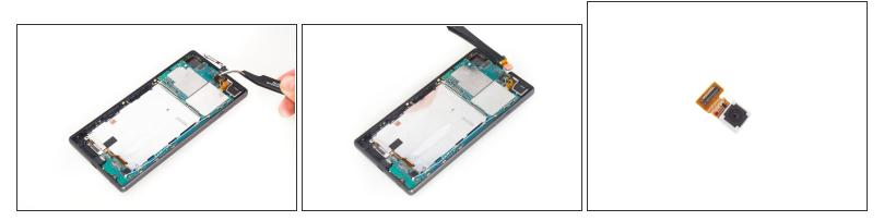
Remove that securing bracket, then remove front camera.
