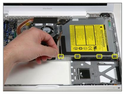
Deroute the hard drive connector cable from the four tabs along the edge of the optical drive.
