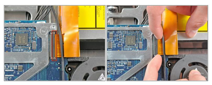
Gently pull the cable retainer on the optical drive cable ZIF socket toward the right side of the iMac.
