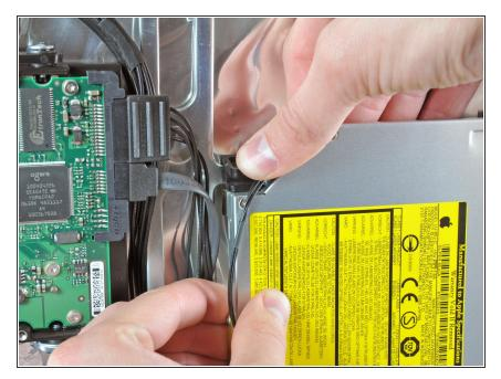
Push down on the optical drive bracket retaining clip while pulling the top edge of the optical drive away from the rear case.
