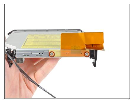
Remove the two T6 Torx screws securing the optical drive cable to the optical drive.
