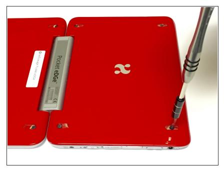
Using your J1 Phillips head screwdriver, remove all eight 6mm screws from the back of your device.
