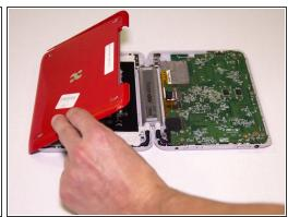
• Using the plastic opening tool, lift the back plate from both sides of your device and remove them.
