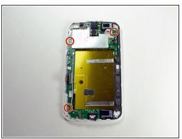
Using a T5 Torx screwdriver, unscrew the three 2.2 mm screws holding the motherboard in place.
