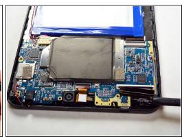
Disconnect the any wires that are connected to the motherboard.
