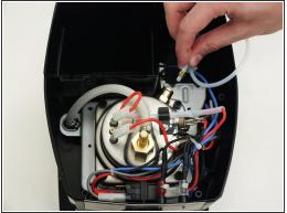
Remove each clip from the valve and core using the precision angled tweezers.
