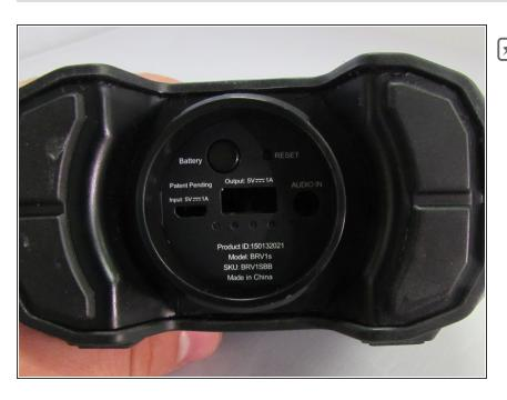
when screwing in the replacement rear water cap, ensure it is properly aligned to ensure the device remains waterproof
