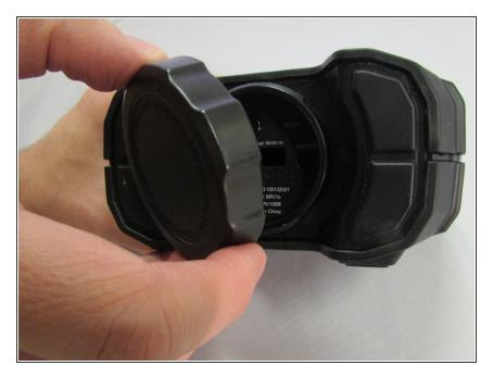
Unscrew the Rear Water cap in a counterclockwise rotation with your fingers
