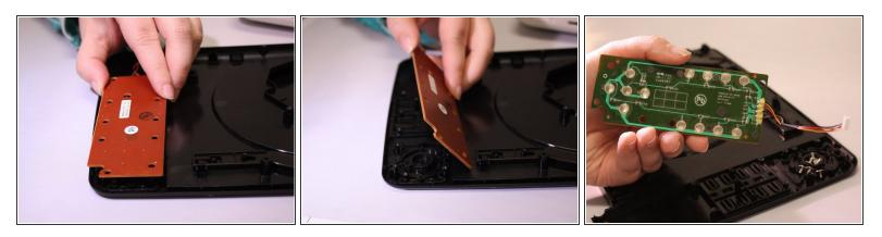
• Once unscrewed. gently pull upwards detaching the button panel from the casing.
