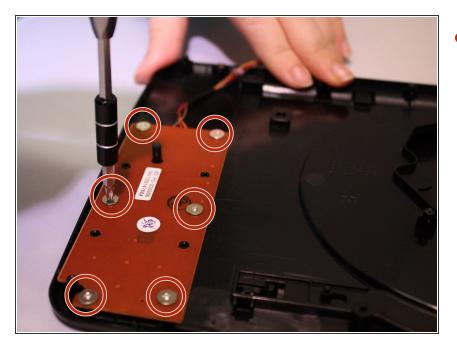
On the bottom side of the disk flap case, the back of the button panel will be visible. Using a Philips J0 screwdriver, unscrew all 6 screws.
