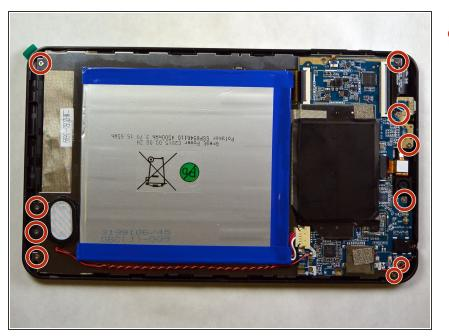
• Remove the 10 JIS #000 screws from the back of the device.
