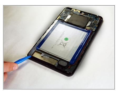
• After removing all of the screws and disconnect any wires, use the blue plastic opening tool and starting from the bottom near the battery, carefully lift the back metal plate and motherboard out. Set aside in a secure place.
