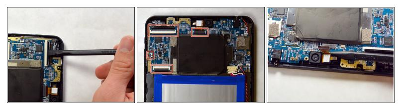
Using a spudger, lift the flaps securing the four ZIF connectors.
