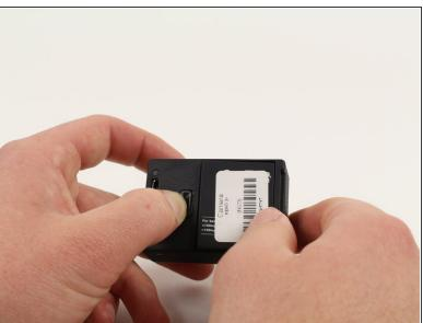
Push the tab on the back of the device left to remove the plate covering the battery.
