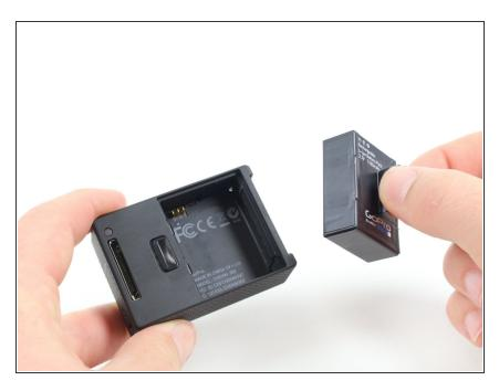
Use the strip of tape on the battery to remove the battery from the housing.
