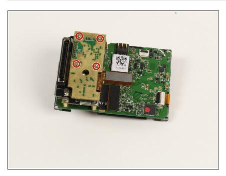
Remove the four 4mm PH00 screws attaching the image sensor to the motherboard with your screwdriver.
