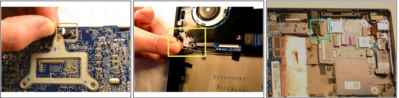
**i** Before removing the motherboard, there are a few cables to disconnect.
